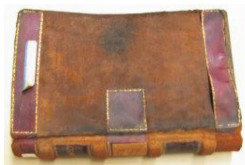
Fig No.2 Leather bound book damaged due to changes in climate and suffered by red rot
